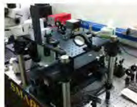
Nanostructure vibration measurement system using optical comb as a light source
