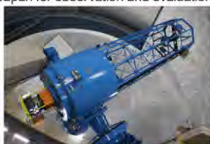
188 cm astronomical telescope equipped with astro-comb
